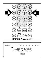
Press and hold (PRI) /TURBO for two seconds to designate this channel as your new Priority Channel.
